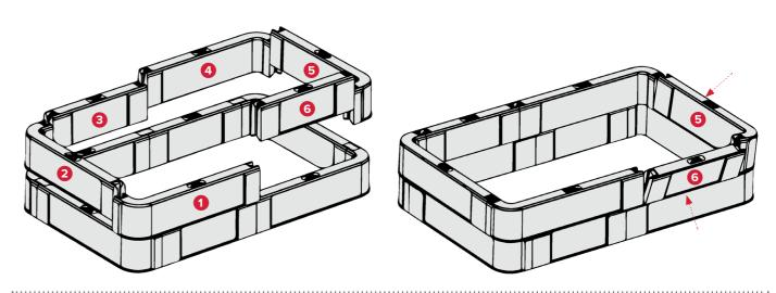
Repeat steps 1 to 3 until the chamber reaches the specified depth.
