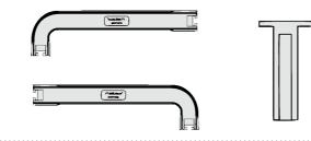
a) Arrange corner pieces to match the chamber clear opening dimensions. Ensure that the lip is on the outside of the chamber. The corner pieces should be all 'left' or all 'right' on each section and will alternate between the two as the chamber increases in depth. b) Connect the sections using jointing pegs, ensuring that the top of the peg is level with the top of the section. All pegs should be partially inserted before tapping.
