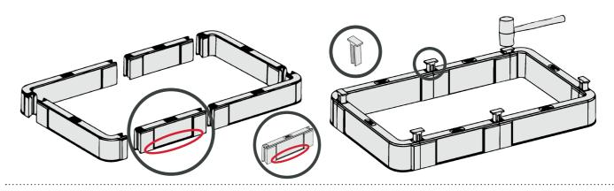
'brick worked' chamber ensuring any joints are not in a vertical line.
