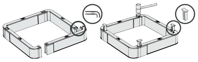
a) Using the alternative corner piece arrangement, lay out the second ring section of connect pieces to ensure you have the correct components. b) Arrange the component parts sequentially as shown below. This will provide a 'brick worked' chamber ensuring any joints are not in a vertical line.
