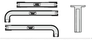
a) Arrange corner pieces and side walls to match the chamber clear opening dimensions. Ensure that the lip is on the outside of the chamber. The corner pieces should be all 'left' or all 'right' on each section and will alternate between the two as the chamber increases in depth. b) Connect the sections using jointing pegs, ensuring that the
