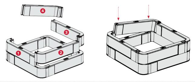
Connect the sections using jointing pegs, ensuring that the top of the peg is level with the top of the section. Repeat steps 1 to 3 until the chamber reaches the specified depth.
