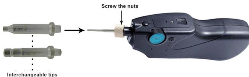
To mate different connectors, various tips are available and interchangeable. Firstly loosen the retaining nut. Then remove the tips along the lens bar. Lastly make the change and tighten back the retaining nut.
