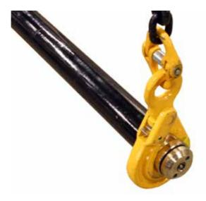
2) Push reel axle through reel's holes. Set axle so that it's positioned at the middle of the axle. Install cones to reel holes and lock them with two-part reel locking bands.
